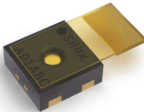
Figure 20. Sketch of the SHT4x with attached polyimide foil.
