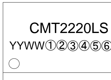
Figure 10. CMT2220LS Top Marking
