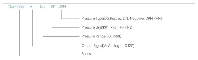
Note: 1. For specific output e.g 0.2~4.9V,signify output figure behind part number, e.g.: XGZP6895A250KPD0249
